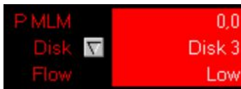
Fig. 4.35: Low – Disk pressure differential is too low
